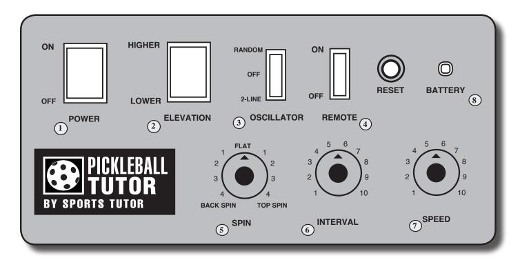
Panel shown with electronic elevation, 2-Line oscillation and remote control options.
